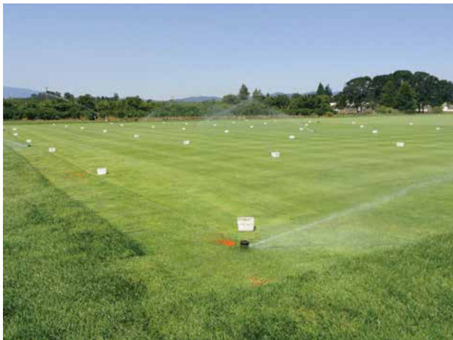
Catch cans (4 inches × 4 inches) were placed across a sand-based putting green every 10 feet × 10 feet to determine the average precipitation rate, low quarter average and distribution uniformity of the irrigation system at Lewis-Brown Farm, Corvallis, Ore. Photo by Brian McDonald
