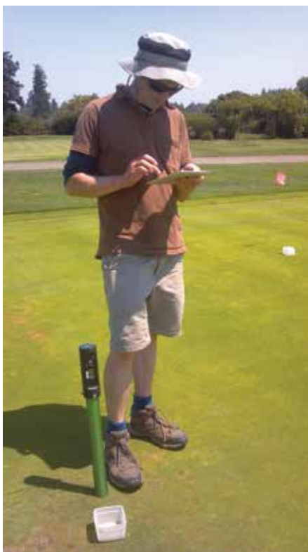
A POGO and an iPad Mini were used to measure the moisture content across a sand-based putting green at Lewis-Brown Farm, Corvallis, Ore. Photo by Alec Kowalewski
