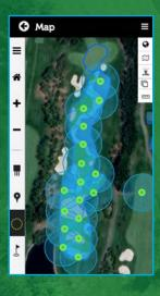
Layer sprinkler patterns over Visual Insight to correlate how sprinkler patterns and traffic flow are contributing to the conditions you measure and see. **TRULY dial in your irrigation system**, perfectly! POGO sees what conditions are associated with each and every station, and clearly indicates *best adjustments to achieve uniform irrigation application while saving time and money*!
