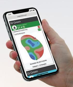
Once enough measurements for a zone have been recorded, anyone on your team can view the analysis, and make the right decision about what to address and where. An average size putting green gets in-depth analysis with only 10-15 samples randomly logged in less than 2 minutes. (FW's and sports fields ~6 to 10 minutes)
